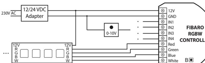
Fig. 10. - RGBW strip with 0-10 V potentiometer wiring diagram
