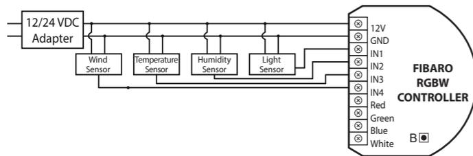
Fig. 8 - 0-10 V sensors wiring diagram
