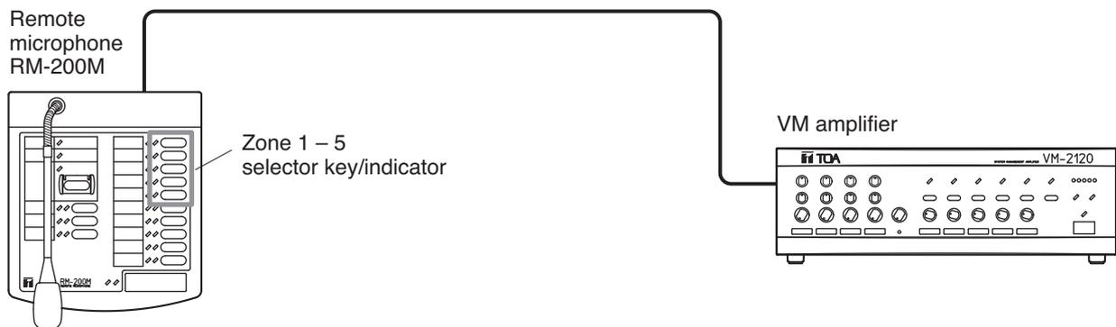
(2) 5 speaker zones with 1 VM amplifier (equipped with the EV-200M Board)
