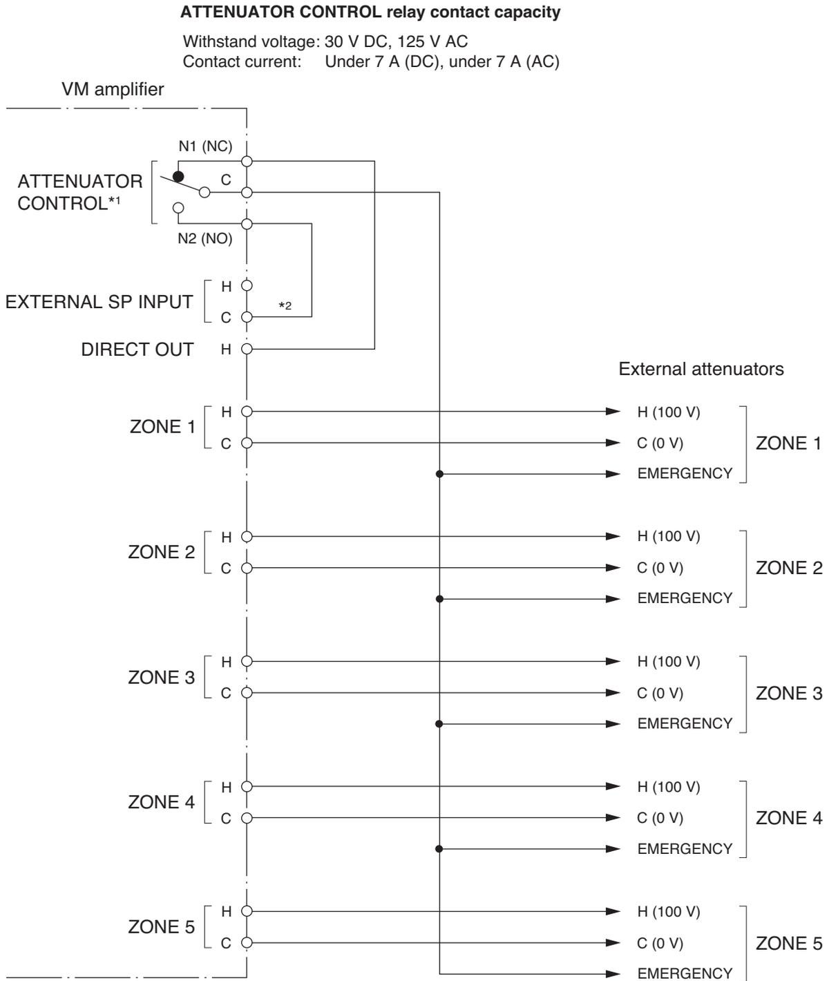
\*1 This figure shows the relay operation status when the VM amplifier's power is switched off, when it is making All-zone or emergency broadcast or when its broadcast is cut off due to control from external equipment in emergency broadcast mode.
