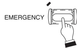
A pre-recorded Alert signal tone and Alert announcement will be alternately broadcast to the entire zone for the preset number of repetitions.\*1 The EMERGENCY indicators of the RM-200M and the VM amplifier come on.
