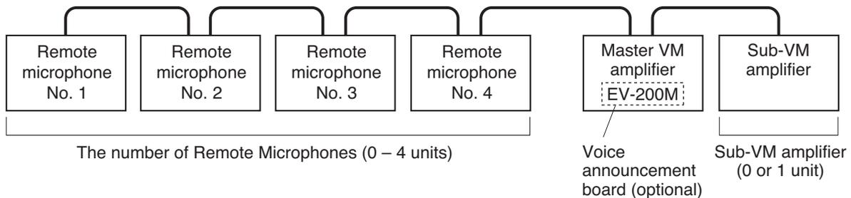
Set the Remote Microphone's Unit number (1 – 4) using DIP switches No. 1 and No. 2 on the microphone's right side panel. The Unit number may be set regardless of the unit's connection order. (See p. 40 "VM Amplifier's Internal Function Switches.")
