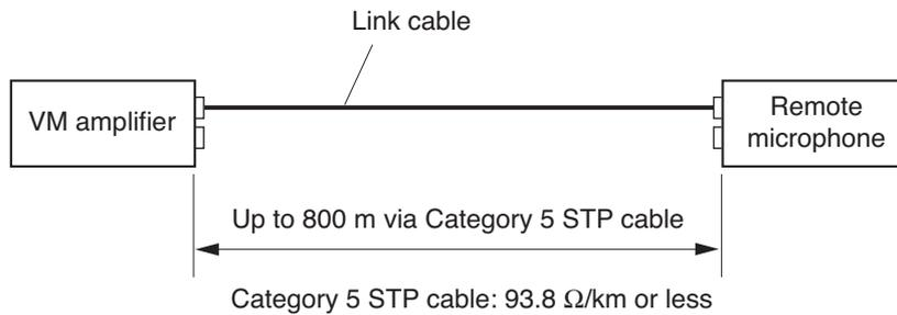
(2) Power supply using cables other than Link cable
