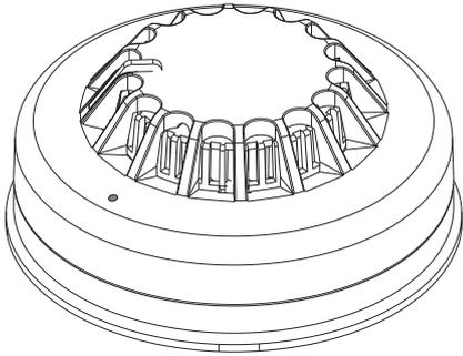
**COPP420 Analogue photoelectric sensor**, this is the most commonly used Sensor and is most suitable for detecting slow burning fires.
