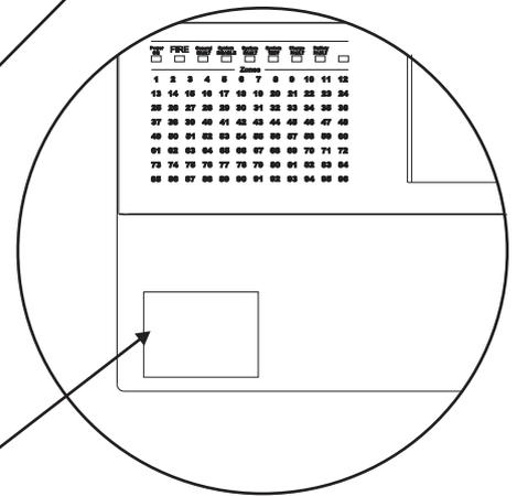
NOTE: If the panel is recessed this label must be placed on the front of the panel as indicated.
