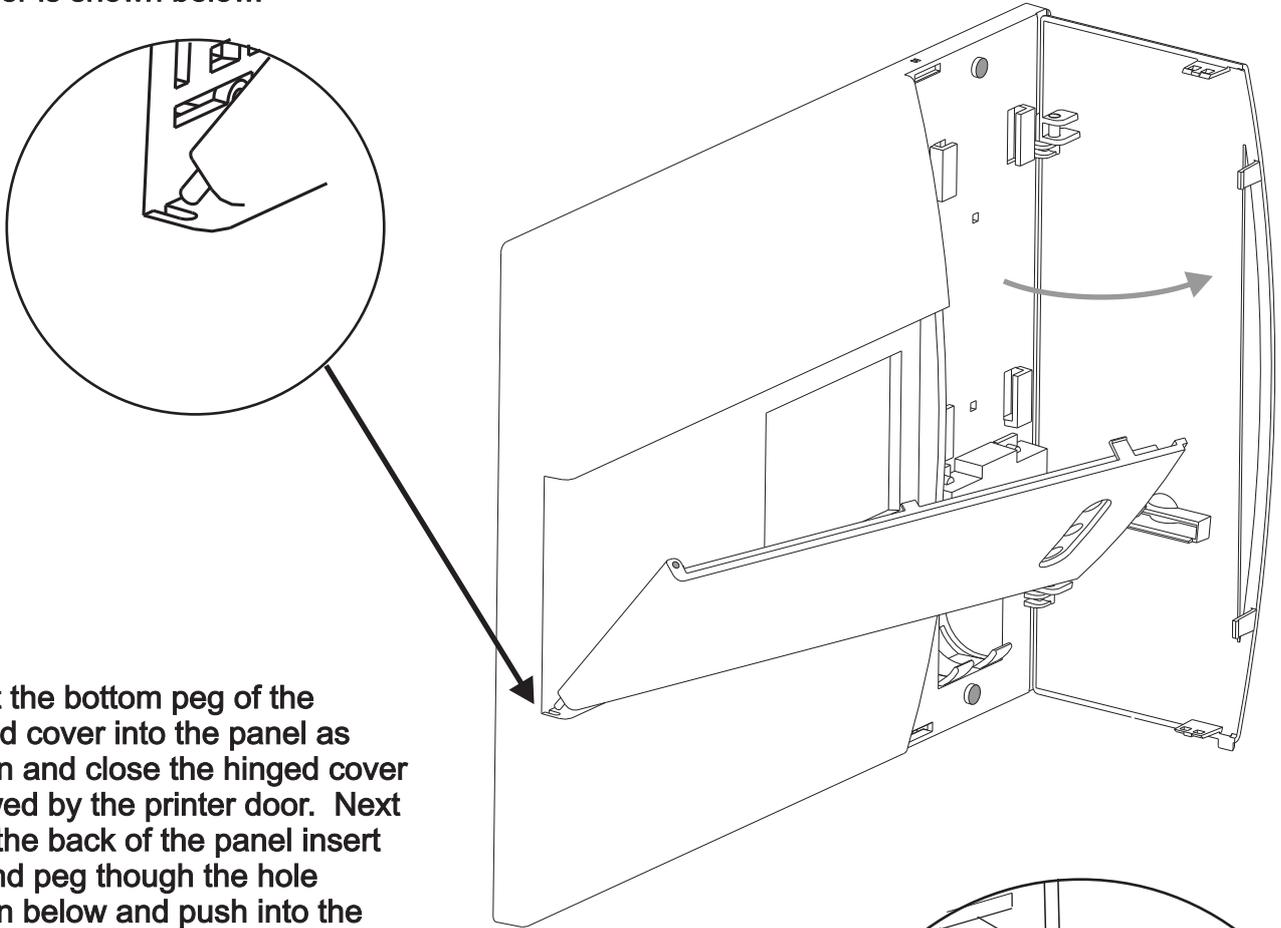
Insert the bottom peg of the hinged cover into the panel as shown and close the hinged cover followed by the printer door. Next from the back of the panel insert second peg through the hole shown below and push into the hinged cover
