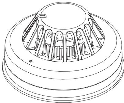
**COPOH450 Analogue photo/thermal sensor**, this is a new addition to the Cooper Fire Systems range of sensors. It is the ideal Sensor for a multi-use environment as it has an excellent response to smouldering and fast burning fires. photo/thermal sensors can be programmed for thermal only operation at certain times of day
