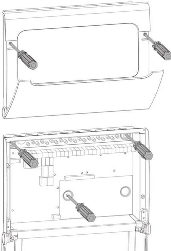
Mount the panel, using pre drilled screw positions, to the wall. This will prevent any possible brick dust contamination of the panel internal circuitry. Use Three No.10 x 1 ¼" (5.0 x 30mm approx.) pan head screws. When using 20mm conduit entry direct to ensure a wide distribution of pressure when tightening the coupling.
