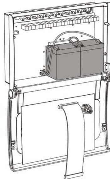
3. Carefully reattach the ribbon cable. The 16 Zone panels have a battery bracket to secure the batteries this should be fitted before reattaching the ribbon cable.
