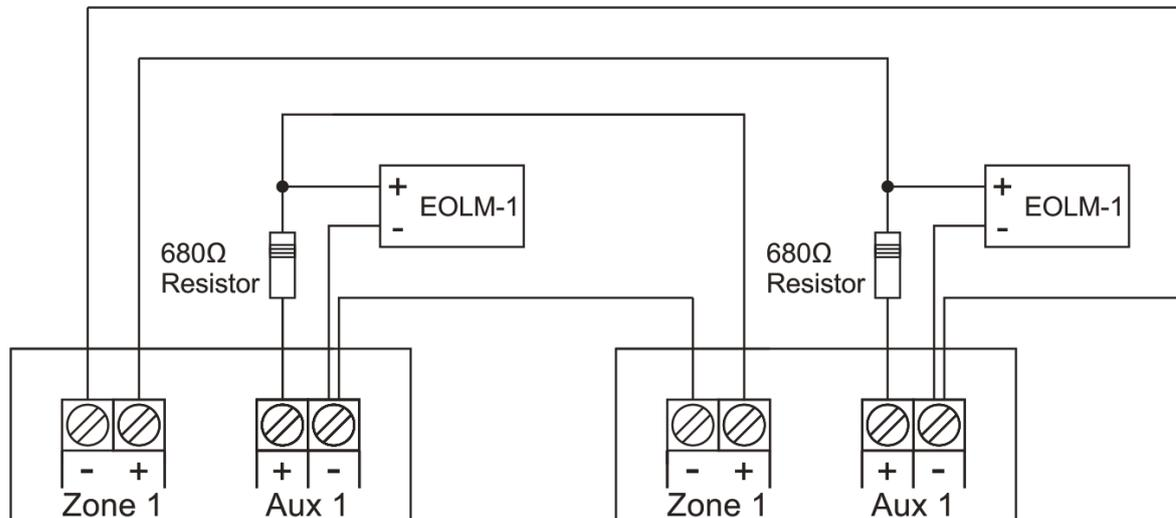
Zone 1 of Panel 1 must be connected to AUX 1 of Panel 2, with an EOLM-1 and 680Ω resistor as shown in the diagram above.
