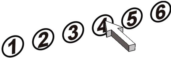
The yellow LED of the zone 1 is flashing. Push button 4 several times until the yellow led of the relevant zone is flashing.
